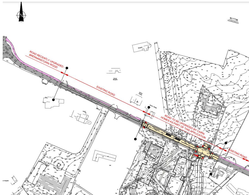
Figure 23 Drawing showing upgrade works to Brennanstown Road
